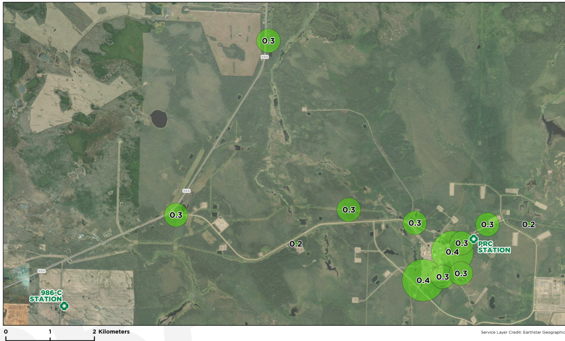
Figure 56: 2023 Annual average sulphur dioxide measured by PRAMP's passive monitoring network (in parts per billion).
