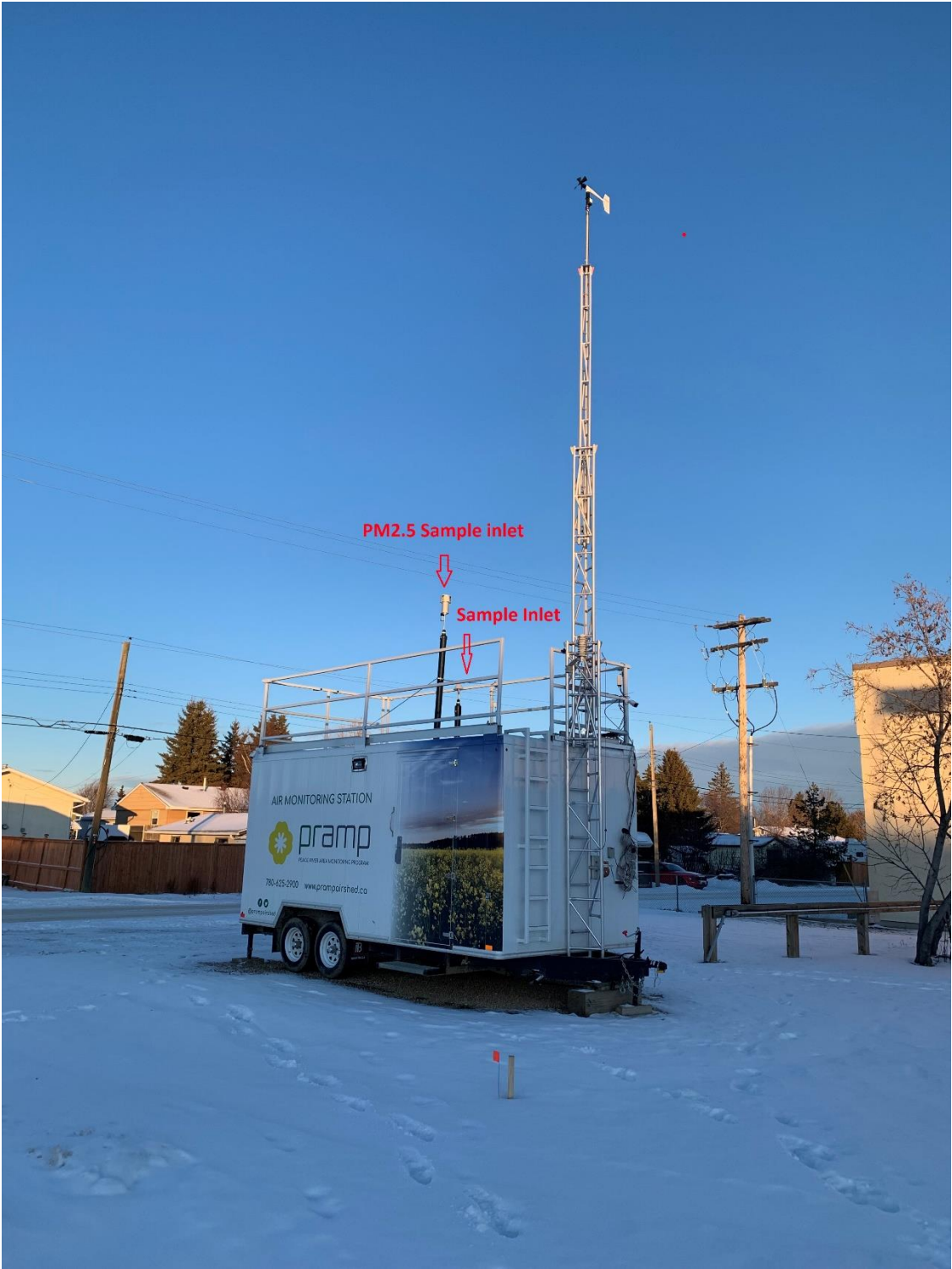
Colour picture showing the details of the sampling inlet(s) or manifold in relation to the station.
