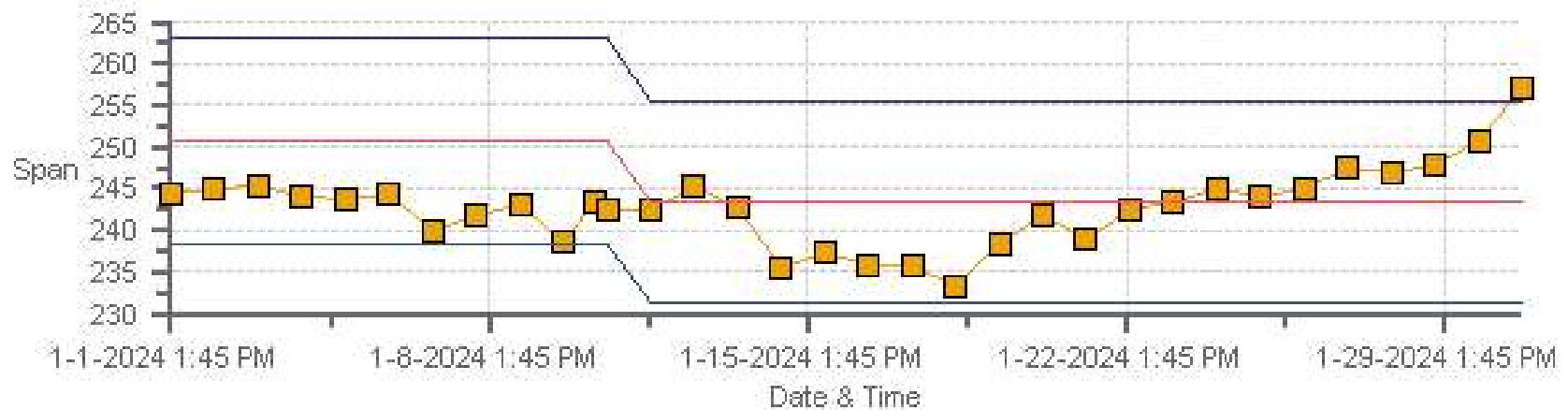
SO2[ppb] Calibration: PRAMP 986-C Monthly: 01-2024 Type: SpanAndZero - Span
