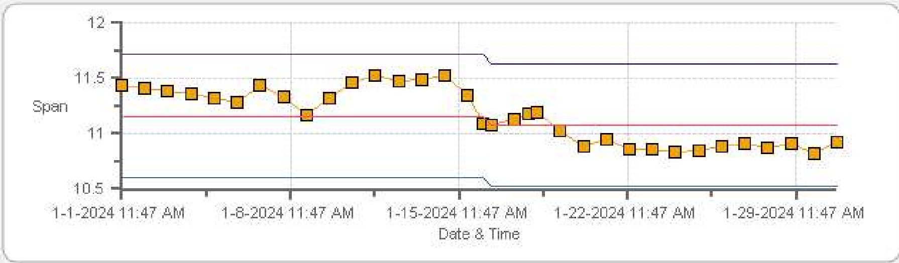
NMHC[ppm] Calibration: AQHI Grimshaw Monthly: 01-2024 Type: SpanAndZero - Span
