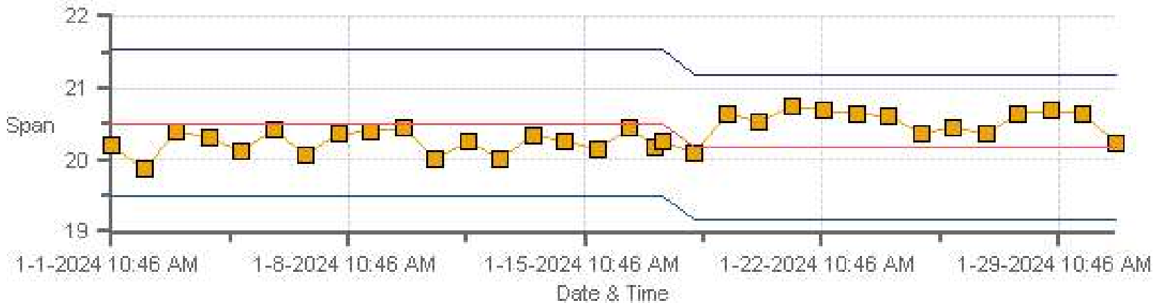
THC55[ppm] Calibration: PRAMP 842-B Monthly: 01-2024 Type: SpanAndZero - Span
