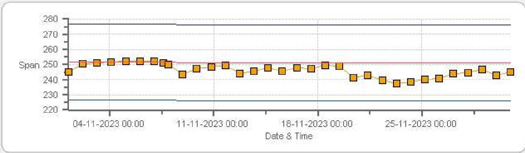
SO2[ppb] Calibration: PRAMP 986-C Monthly: 11-2023 Type: SpanAndZero - Span
