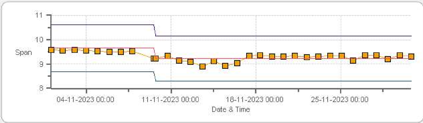
CH4[ppm] Calibration: PRAMP 842-B Monthly: 11-2023 Type: SpanAndZero - Span
