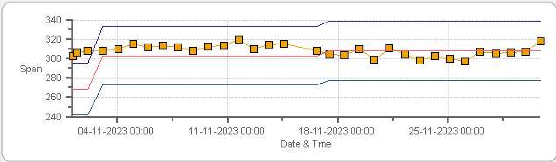
NOX[ppb] Calibration: AQHI Grimshaw Monthly: 11-2023 Type: SpanAndZero - Span
