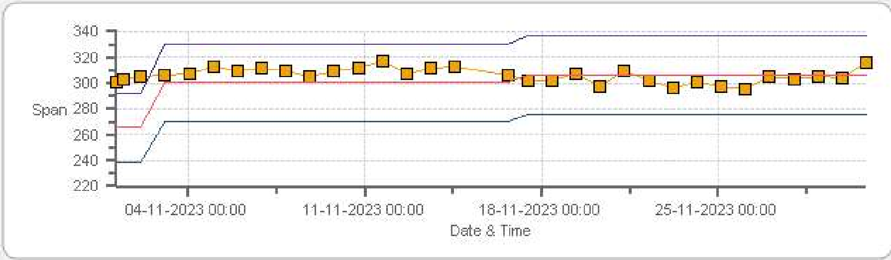
NO2[ppb] Calibration: AQHI Grimshaw Monthly: 11-2023 Type: SpanAndZero - Span
