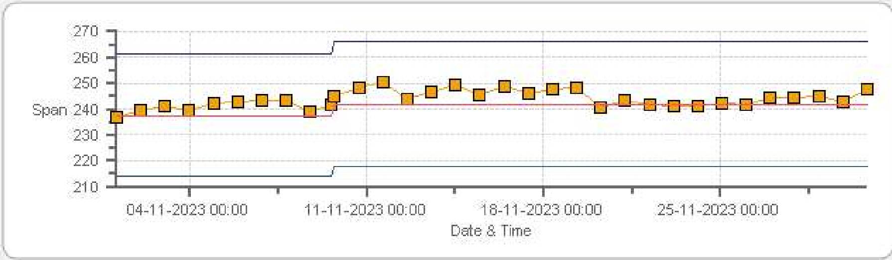
SO2[ppb] Calibration: PRAMP 842-B Monthly: 11-2023 Type: SpanAndZero - Span
