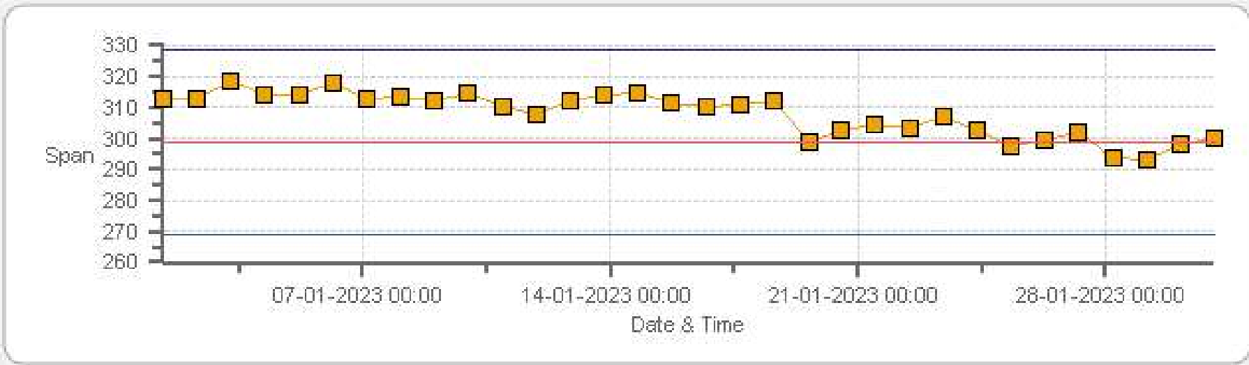
NO2[ppb] Calibration: AQHI Grimshaw Monthly: 01-2023 Type: SpanAndZero - Span
