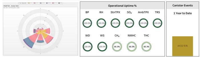
**Operational Summary\_THC/CH**<sub>4</sub>/**NMHC**: Uptime was 66.3% = 251 hrs of downtime (AEP reference # 346425). Shut-down calibration on Oct 31 did not meet stability requirements due to poor injections. Data discarded back to the point of failed performance on Oct 21 @ 06:00 (-251 hrs). Canister: No events recorded this month.
