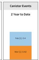
Operational Summary\_TRS: Uptime was 99.7% = 2 hrs of downtime. 2 additional zero-span checks (IZS) were performed on Jul 3 & 4 to assess a biased low span response. THC/CH<sub>4</sub>/NMHC: Uptime was 98.9% = 8 hrs of downtime. Low carrier gas pressure on Jul 2. Cylinder was exchanged followed by an additional IZS (-7 hrs). Manifold cleaning on Jul 4 (-1 hr.) Canister: A 5-min conc. of 2.10 ppm was recorded on Jul 2, while the carrier gas was replaced. Not considered a real event.
