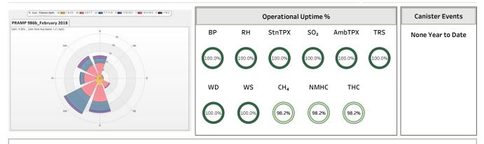
**Operational Summary\_THC/CH**<sub>4</sub>/**NMHC**: Uptime was 98.2% = 12 hrs downtime. Due to low fuel gas pressure the analyzer recorded anomalously low hourly and span data on Feb 7. The fuel gas cylinder was replaced, followed by a zero-span check (-10 hrs). Following monthly calibration on Feb 15, the channels remained offline in order to test the canister trigger program on the Ultimate datalogger (-2 hrs).
