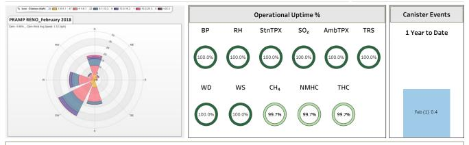
**Operational Summary\_THC/CH<sub>4</sub>/NMHC**: Uptime was 99.7% = 2 hrs downtime. The fuel gas cylinder was replaced on Feb 9, followed by a zero-span check (-1 hr). The sample manifold was cleaned prior to the start of monthly calibration on Feb 22 (-1 hr). A canister event was recorded on Feb 25 at 23:50, at an initial conc. of 0.40 ppm.
