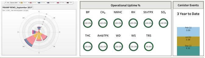
**Operational Summary\_TRS**: Uptime was 99.6%, equivalent to 3 hrs downtime. The monthly calibration was performed on Sept 19. The first attempt was aborted due to an operator transcription error that yielded incorrect adjustments. The analyzer was reset to the as-found state and the second calibration attempt was successful. NMHC: Canister event triggered on Sept 7 @ 20:00 (0.32 ppm).
